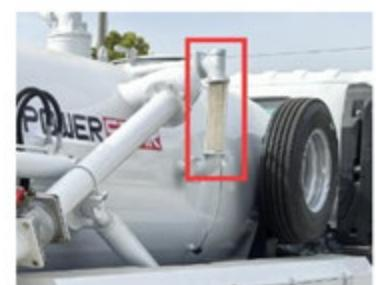
**Note:** 1) Only suggest use vacuum pump for Pump-In working, strictly forbidden for Pump-Out working;
